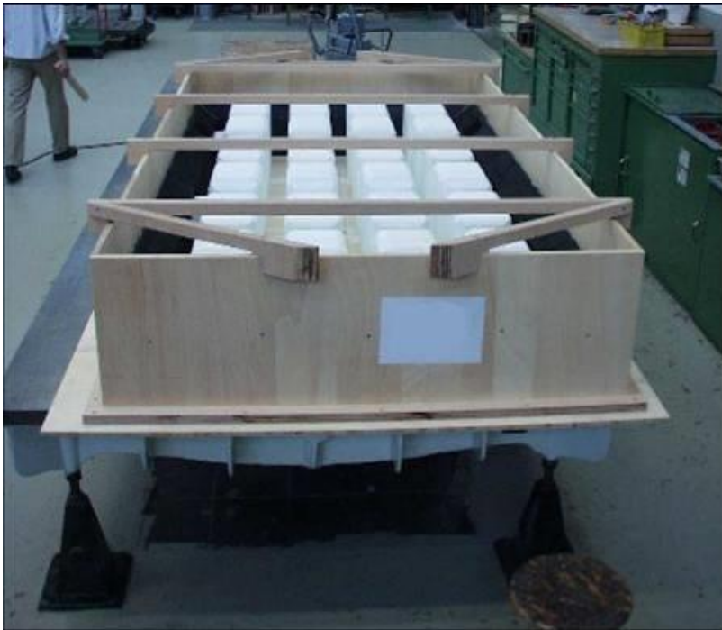
car roof - mold
