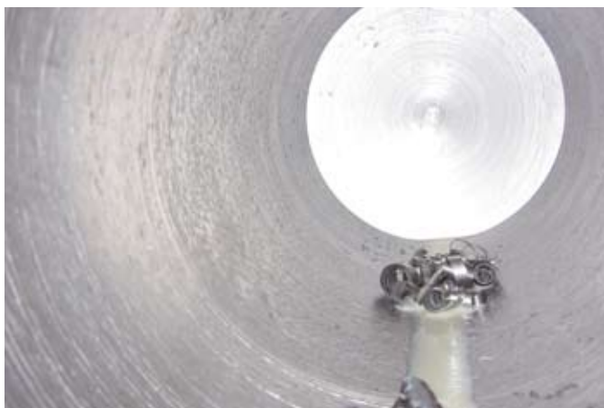
Application example: Drilling into the solid with \varnothing 185.00 mm in material 34 CrNiMo with 1000 N/mm 2
