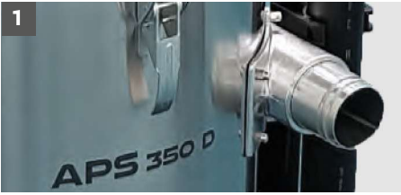
1 Tangential inlet Cyclonic effect separation
