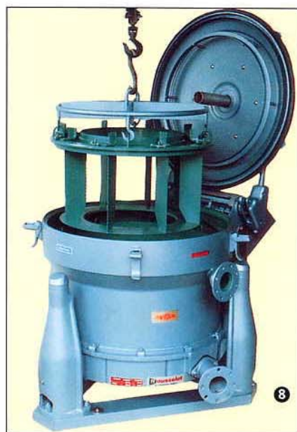
Centrifugal Decanter with removable cage for solids removal, and liquid phase removal being achieved by overflow
