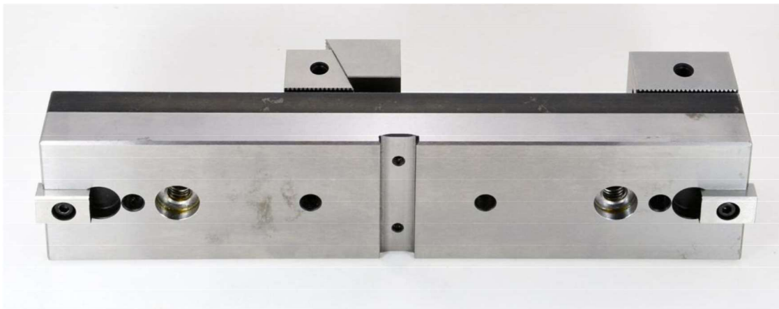
PSE clamping rail 320 mm prepared with notches 16 H7 mm and fitting bores \varnothing 25 H7 mm screwing through T notch 4 times distance 80 mm for M8 screws
